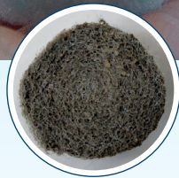
Cross-sectional area FIBALON® (used)
